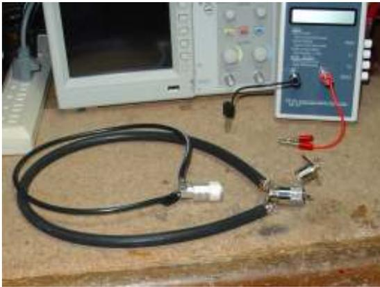
Photo C: Ferrite choke measuring loops
